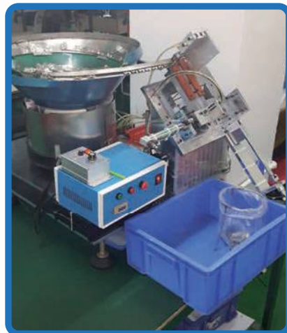
彈片平整度檢測 / 校正儀 Flatness analyzer for battery clips
